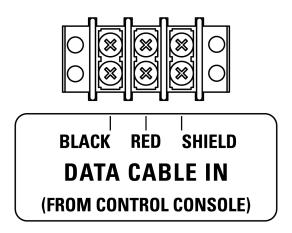
You may purchase data cable from Electro-Mech, or you may source it elsewhere. We recommend (and supply) cable that is rated for direct burial. It includes two insulated 22 AWG stranded conductors (red and black), along with a non-insulated conductor, all wrapped by a braided or foil shield. This document will discuss, in a few pages, what the other end of this cable is connected to.
